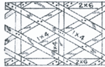
LATTICE PURLIN OR TRUSS
